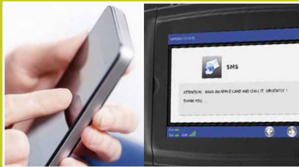
GSM Kit to send SMS alerts about the status of the machine to the user's cell-phone and to receive messages from the user's cell-phone
